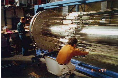
Figure 2.4: Drift Chamber during wire stapling
