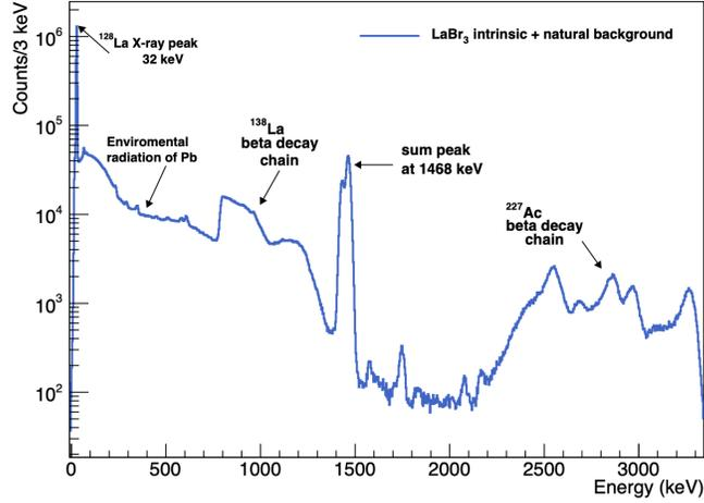
Figure 2: *Background spectrum acquired without beam. This spectrum is compatible with the  $\text{LaBr}_3$  intrinsic background spectrum produced by the radioactive isotope  $^{138}\text{La}$  and by the radioactive contaminant  $^{227}\text{Ac}$ .*
