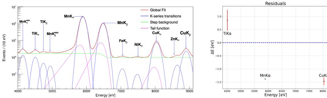
Figure 2: a) Final calibration spectrum given by the sum of all the calibrated spectra of each SDD; b) Distribution of the residuals of the energy of the  $\text{TiK}_\alpha$ ,  $\text{MnK}_\alpha$ , and  $\text{CuK}_\alpha$  lines from their nominal energy. Adapted from <sup>24)</sup>.
