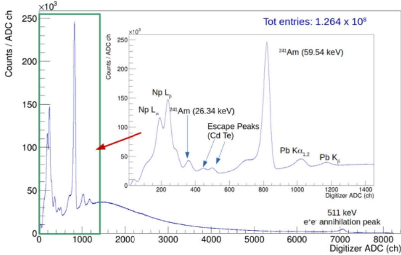
Figure 3: Spectrum collected with the CZT detector and the DAΦNE beam on during the test described in <sup>10</sup>). The annihilation peak at 511 keV and the two peaks coming from the lead shielding scintillation are visible together with the Americium source spectrum. In the box a zoom on the source's peaks around 26 keV and 60 keV is reported.
