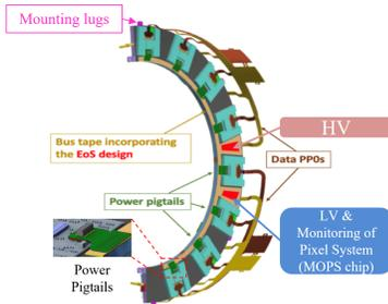
Figure 9: *Half-Ring with pixel modules and services*
