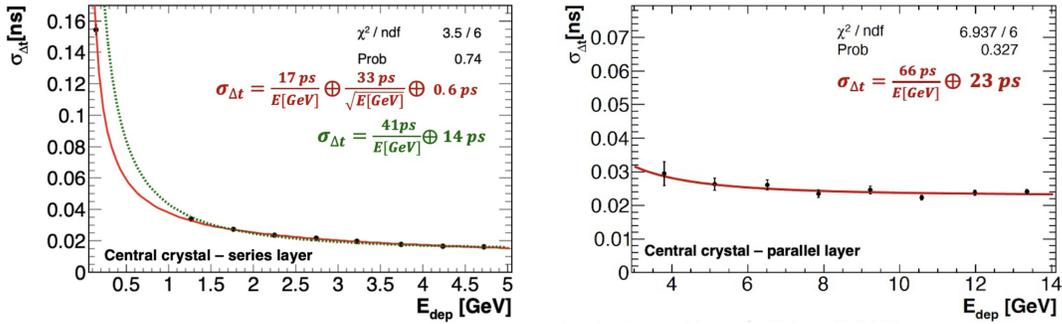
Figure 1: *Proto-1* time resolution as a function of the energy deposit in the most energetic crystal of the layer, for the series read-out module (left panel) and the parallel read-out module (right panel). For the series layer, a time resolution measurement with a 450 MeV electron beam was added and included in the solid-red line fit.
