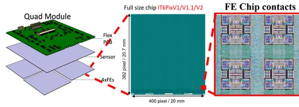
Figure 8: *Quad module with Front-End readout chip*
