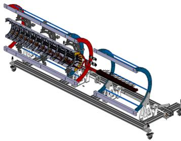
Figure 10: *End-Cap HRs loaded Half-Shell layer with trolley.*
