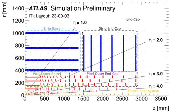
Figure 2: One quarter of the ITk pixel layout
