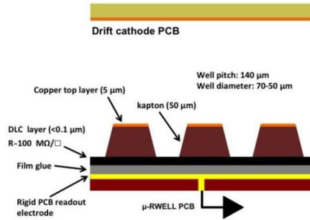
Figure 4: *Layout of the Resistive  $\mu$ RWELL*
