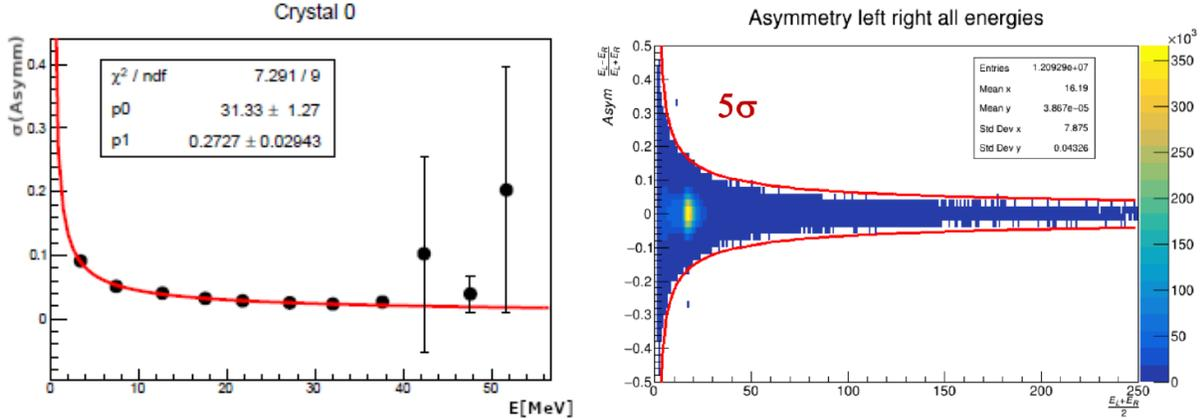
Figure 3: Left:  $\sigma(\text{Asymm})$  distribution of the asymmetry variable for every 5 MeV slice fitted with Eq. 3. Right: The asymmetry variable as a function of the mean energy readout by the two SiPMs. The red lines identified  $5\sigma$ 's described by Eq. 3 for a LY value of 30 photoelectrons/MeV and a SigNoise value of 0.3 MeV.
