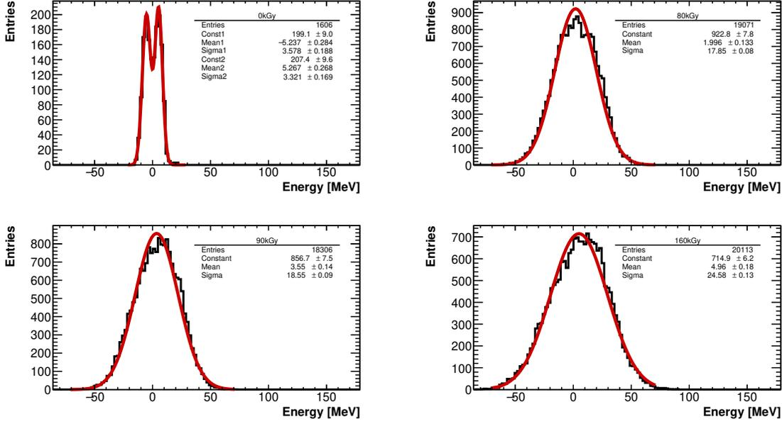
Figure 3: *SiPMs pedestals for read-out channel 11 for different datasets: step I (top left), step II (top right), step IV (bottom left) and step V (bottom right). The dose rates reported in the histograms refer to the SiPM board. The widening of the energy distribution is associated with the increase in SiPM dark counts as the absorbed radiation dose increases.*
