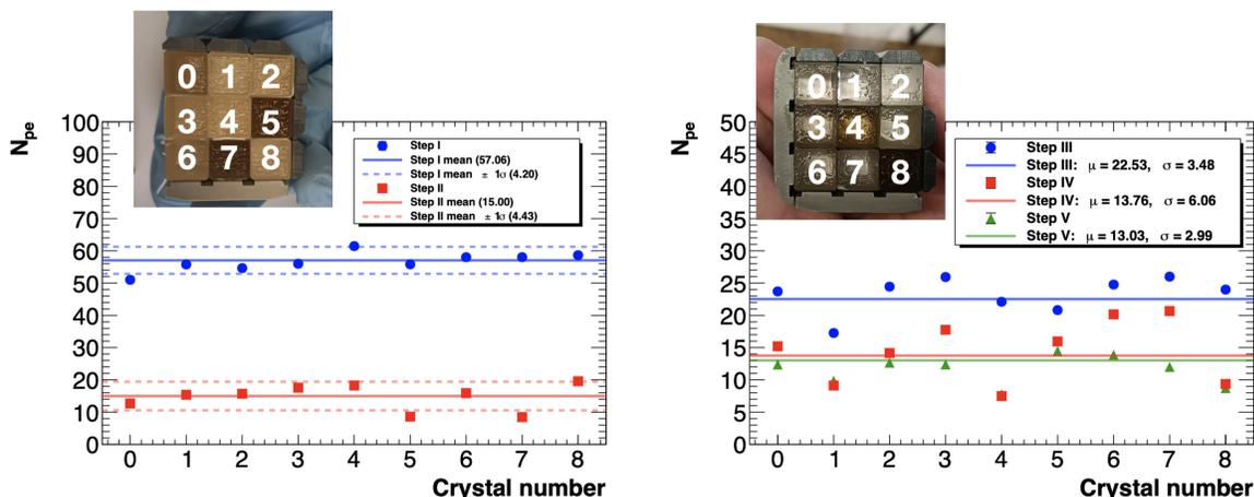
Figure 2: *Left panel: number of photo-electrons estimated for each crystal in the runs with Teflon wrapping (steps I and II). Right panel: number of photo-electrons estimated for each crystal in the runs with Mylar wrapping (steps III, IV and V). The  $\mu$  and  $\sigma$  of the distributions were obtained by a Gaussian fit of the data points. For both cases, a picture of the crystal matrix after the test was included to show the visible transmittance loss and the crystal enumeration choice.*
