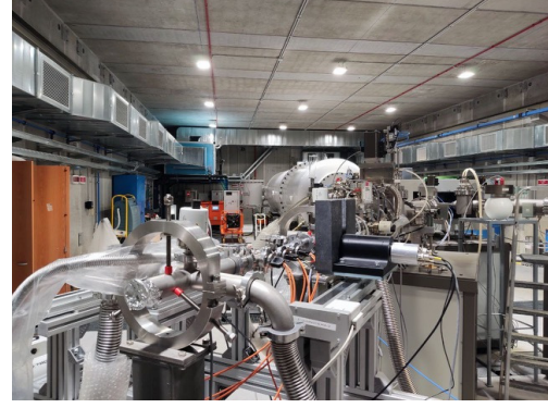
Figure 1: On the left the scheme of the experimental setup for the SHADES gas target. A \text{LaBr}_3 scintillator on a movable table on one side of the target chamber surrounded by lead shielding. On the right a photo of the experimental setup at the Bellotti Ion Beam Facility.
