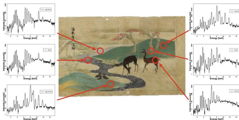
Figure 5: *microXRF spectra of the sampled points obtained by RXR.*
