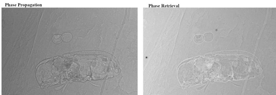
Figure 20: *Phase contrast and phase retrieval radiography for organic sample entrapped in amber. The source parameter are 40 kV, 50  $\mu$ A, 5  $\mu$ m anode focus, distance  $R_1=30$  mm, distance  $R_2=750$  mm and Time acquisition of 1min 30s.*
