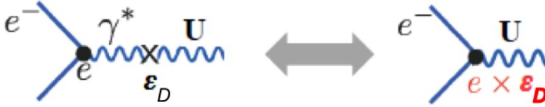
Figure 1: The U boson can communicate with the SM through a kinetic mixing term describing the interaction of the U boson with SM photon. In this case the parameter \epsilon_D should be smaller than 10^{-2} .
