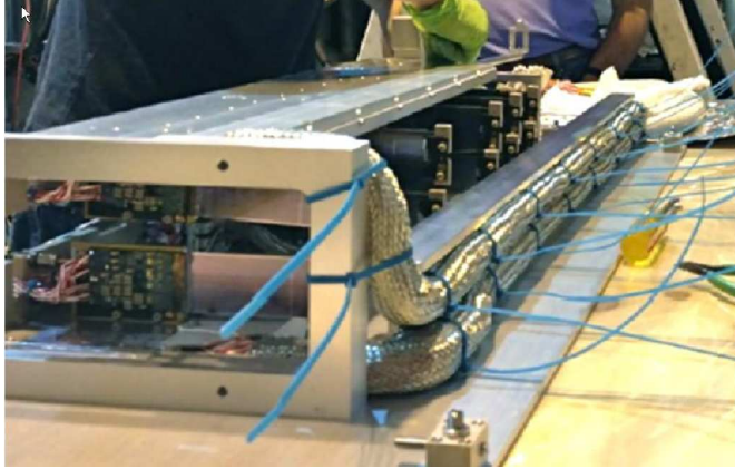
Figure 3: The HPS Test Run silicon vertex tracker, looking upstream. The structure is split top-bottom.
