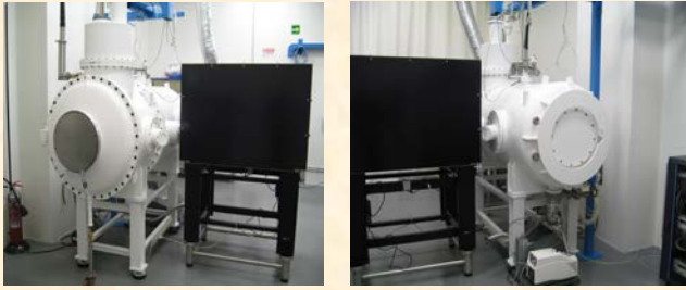
Front and rear view of SCF cryostat. The optical instrumentation is in the black enclosure.
