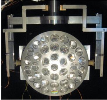
**Figure 1. LAGEOS Sector inside the SCF on the positioning system**
