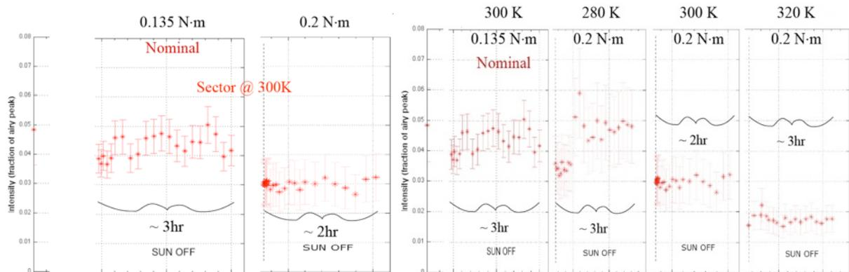
**Figure 4. Effect of polar CCR screw torque (left) and on Aluminum temperature (right) on FFDP intensity after SUN ON phase. Relative error is  $\pm 10\%$**
