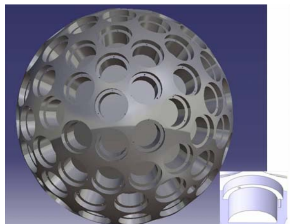
Fig. 5 - LARES satellite with cylindrical cavities.
