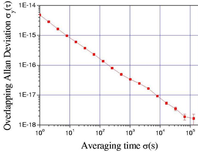
Figure 1: *Fractional frequency stability of the compensated 86 km link.*
