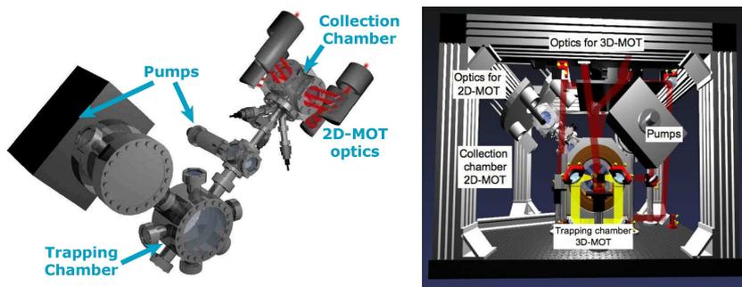
Figure 2: **Left:** *Artist's impression of the ICE vacuum system. Atoms are transferred from the collection chamber, using a 2D-MOT, to the trapping chamber, where they are collected in a 3D-MOT and an optical-dipole trap (FORT).* **Right:** *The ICE mechanical structure with optics and light paths represented.*
