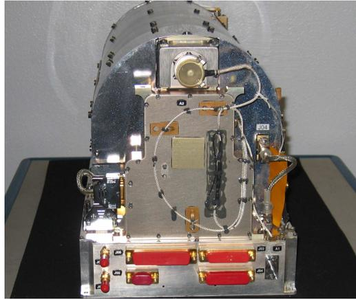
*Figure 2: The PHM is the master clock of the Galileo navigation payload. It is produced by Galileo Avionica (I), that is responsible for the clock performances and produces its electronics, in cooperation with Temex Neuchatel Time (CH), that provides the PHM physics. The PHM design privileges frequency stability and exhibits an excellent frequency drift.*
