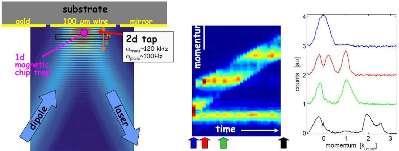
Figure 2: (left) *An optical lattice close to the chip surface by Reflecting a far detuned laser beam from the chip surface creates an optical lattice.* (right) *Bloch oscillations observed in the optical lattice close to the atom chip surface*
