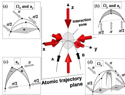
Figure 1: *6-axis inertial sensor principle. The atomic clouds are launched on a parabolic trajectory, and interact with the Raman lasers at the top. The four configurations (a)-(d) give access to the 3 rotations and the 3 accelerations.*
