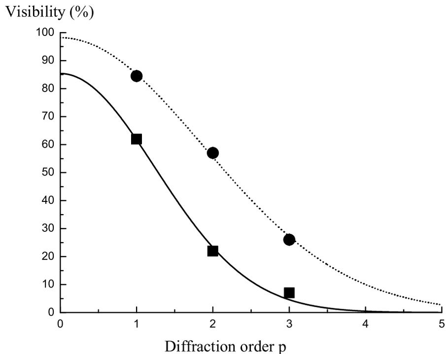
Figure 1: *Fringe visibility as a function of the diffraction order  $p$ . Our measurements (round dots) and those of Giltner et al. <sup>3</sup> (squares) are well fitted by Gaussian functions of the diffraction order  $p$ .*
