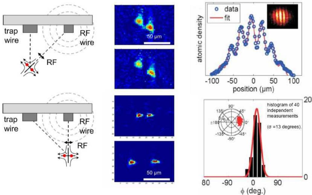
Figure 1: *Splitting an trapped atomic cloud with RF induced double well potential. (left) The orientation of the RF defines the orientation of the splitting. (right) The two split clouds interfere with a stable narrow phase distribution.*
