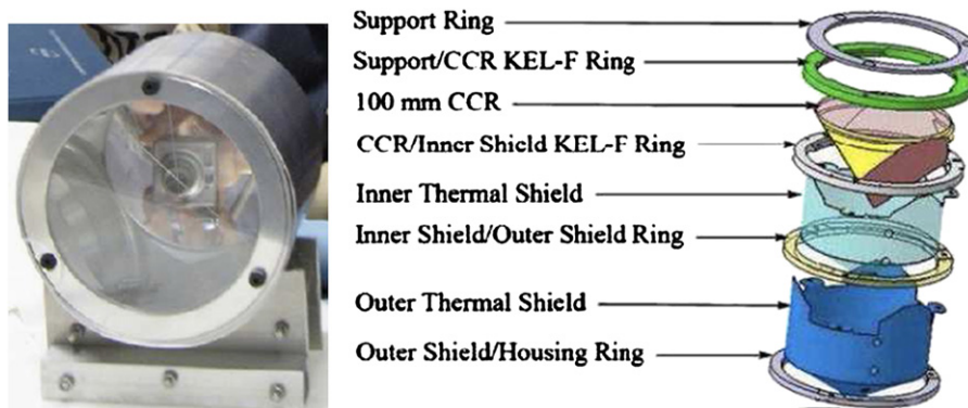
Fig. 5. Views of current design of the MoonLIGHT/LLRRA21 CCR: (a) fully assembled and (b) exploded view with its internal mounting elements and outer aluminum housing.
