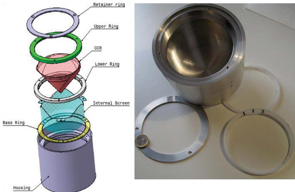
**Figure 4.** Illustration (photo) of 2<sup>nd</sup> (1<sup>st</sup>) CCR housing built at LNF show at left (right). The lower ring (to be made of KEL-F plastic) has line inserts (in black) to reduce heat flow from the cavity to the tabs of the CCR. This is an improvement of the Apollo and LAGEOS design.
