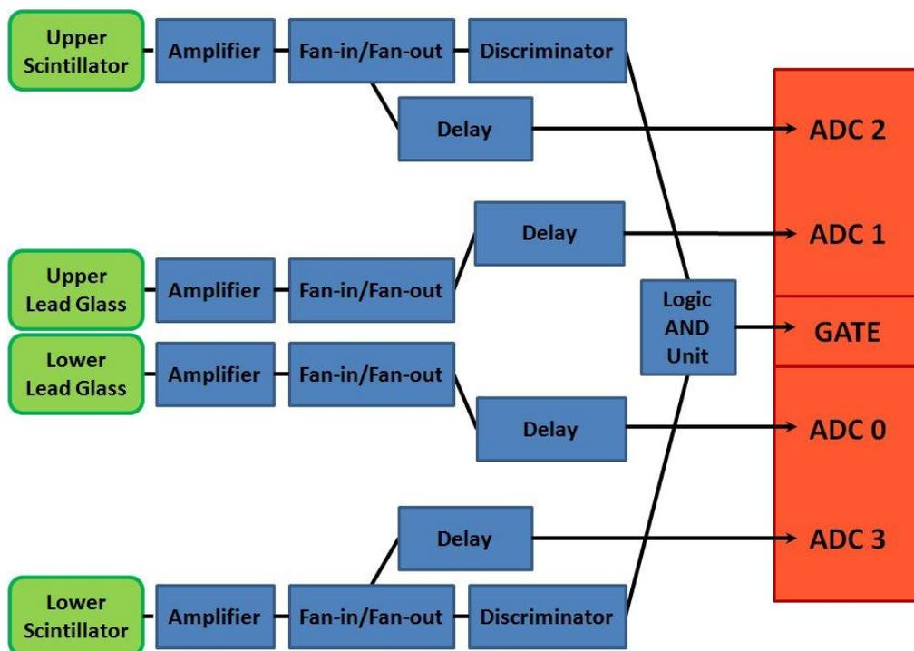
The scintillators are amplified by a factor of 10 and sent to two different fan in/fan out (FI/FO) inputs. We made the gate of the ADC by sending one out of the two FI/FO of the scintillators to discriminators (upper scintillator threshold is 31 mV, lower scintillator one is 66 mV) and the out of these modules to the input of the logic And Unit.
