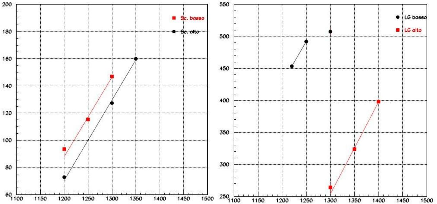
From these curves we calculated the voltages necessary in order to have lead glasses peaks at around 400 and scintillators peaks at around 140. These voltages are:
