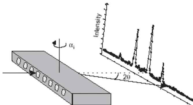
Fig. 2. Sketch of the experimental setup used to measure the far-field pattern of the waveguide grating.
