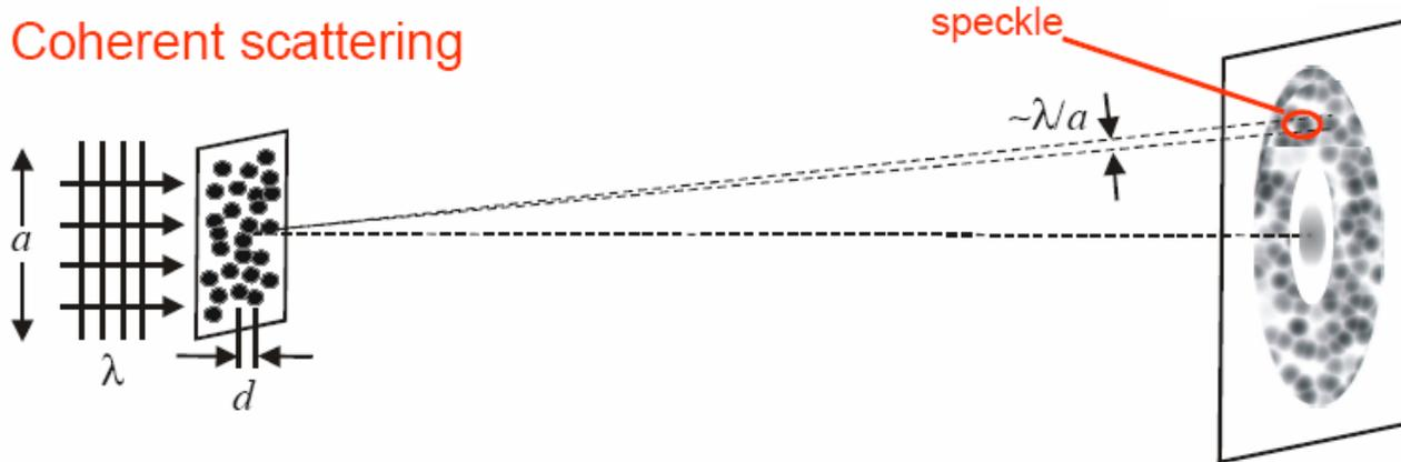
Result of an interference process of the beams diffracted from each single object. The typical 'speckle' pattern contains the spatial information on the single scattering object.
