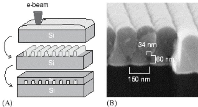
Fig. 1. (A) Sketch of the fabrication process. (B) Scanning electron micrograph (SEM) of the calixarene grating after evaporation of silicon.
