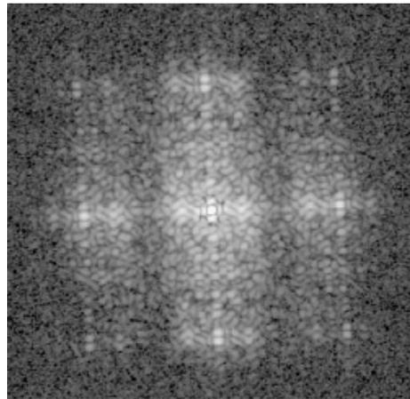
(b) Coherent diffraction pattern from (a)
