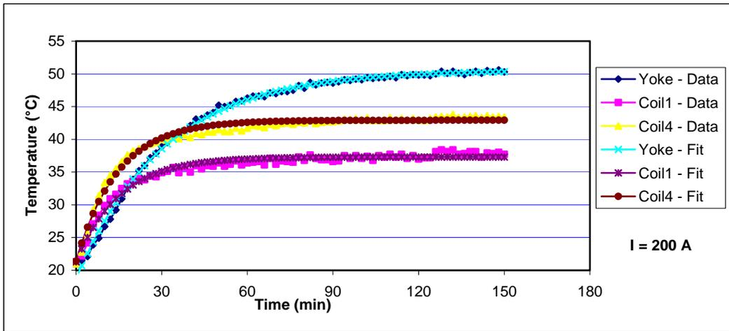
Figure 3: Temperature increase with  $I = 200$  A
