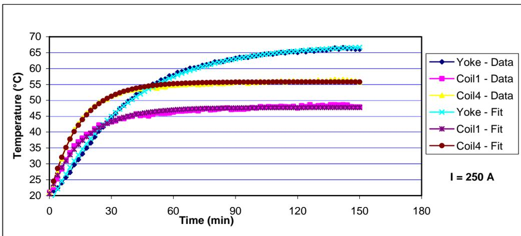
Figure 4: Temperature increase with  $I = 250$  A
