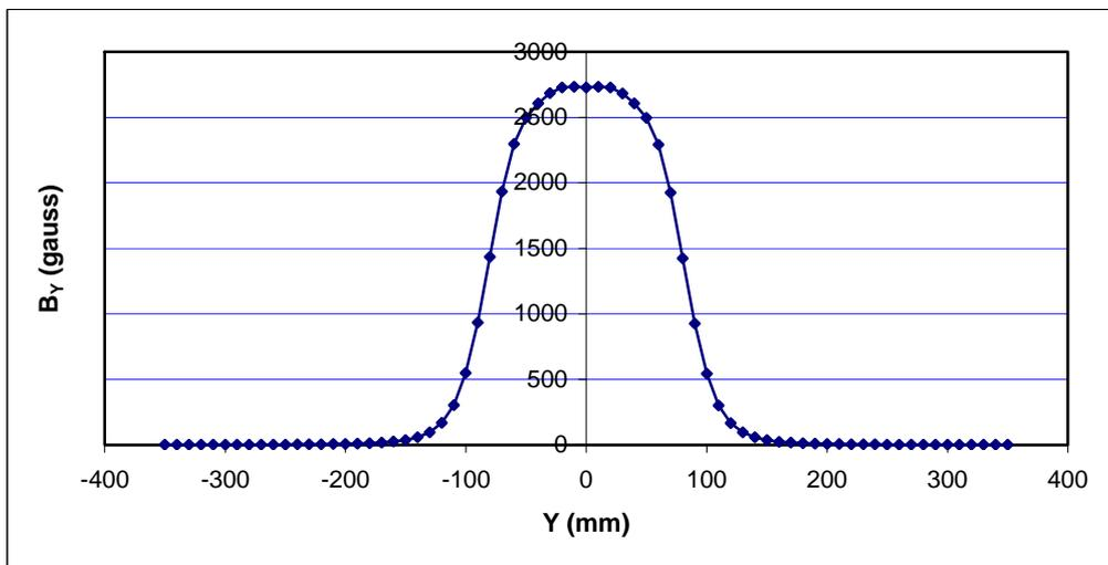
Figure 10: Longitudinal profile of the axial ( $B_Y$ ) component of the field –  $I = 140 \text{ A}$
