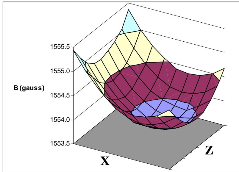
**Figure 7: Example of 2D scanning of the field – Coil B in “single mode”**
