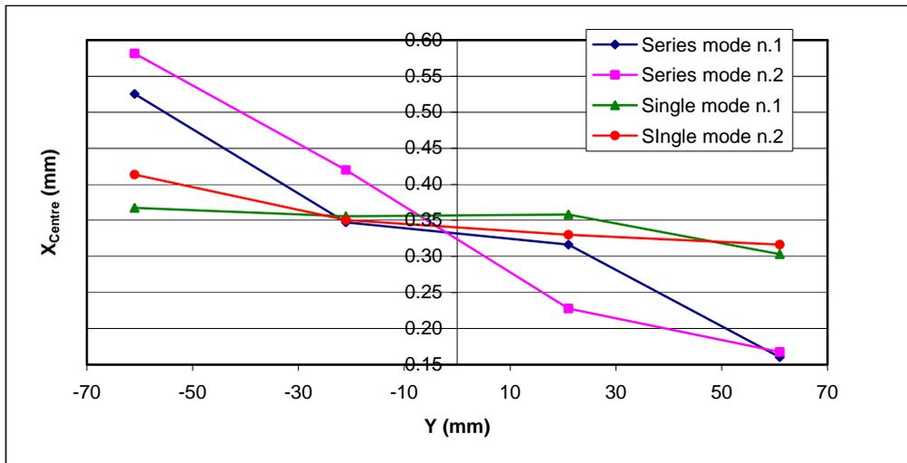
Figure 8: Comparison of the  $X_{\text{Centre}}$  values measured with coils operated in single and series mode.
