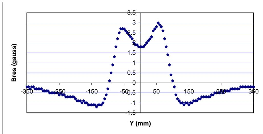
Figure 6: Residual field on the solenoid mechanical axis.
