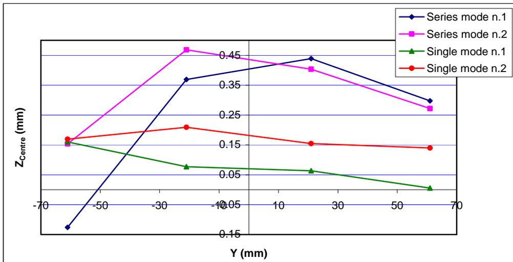
Figure 9: Comparison of the  $Z_{\text{Centre}}$  values measured with coils operated in single and series mode.
