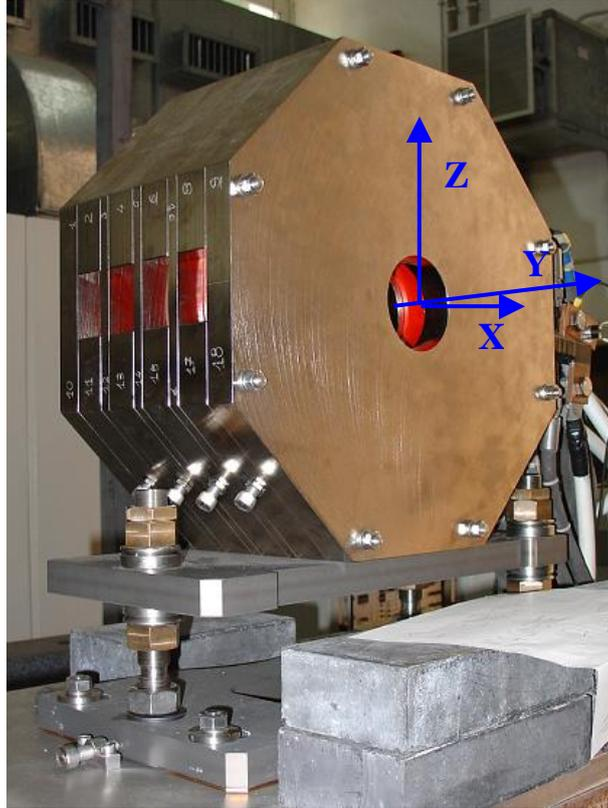
Picture 2 : Reference system for the hall probe measurements of the solenoid.
