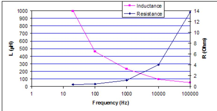
Figure 1: Gun focusing solenoid resistance and inductance versus frequency
