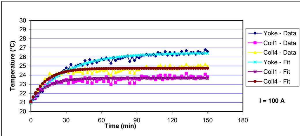
Figure 2: Temperature increase with  $I = 100$  A
