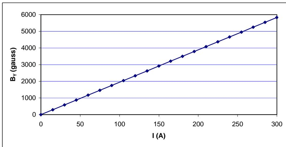
**Figure 5: Longitudinal component of the magnetic field in the solenoid centre (with systematic error on the vertical position) as a function of the excitation current**
