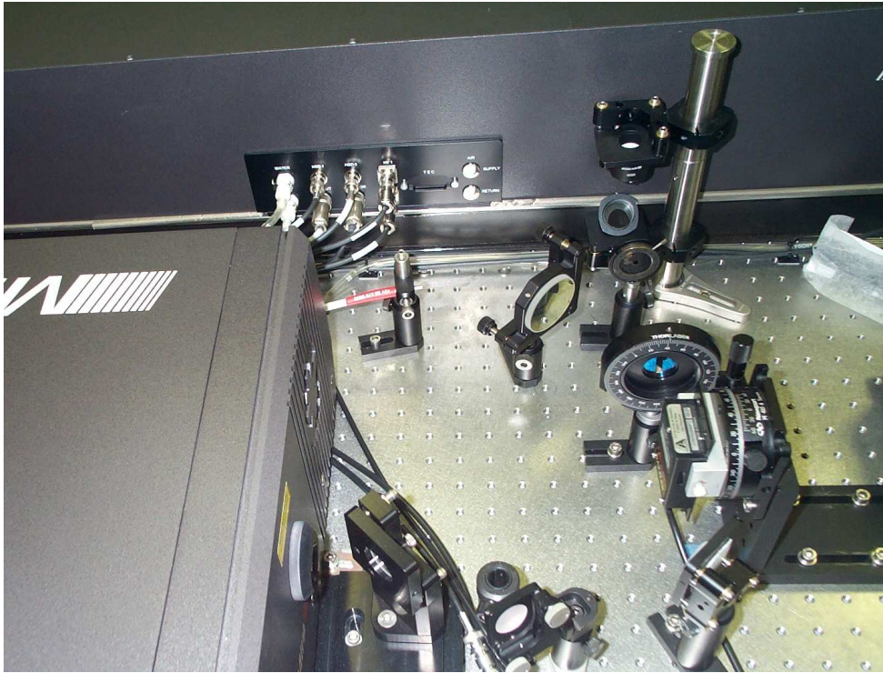
Figure 2. Dazzler set-up: the oscillator output is sent to the acousto-optic filter and a half wavelength wave-plate. After, a periscope is used to inject the beam in the amplifier.
