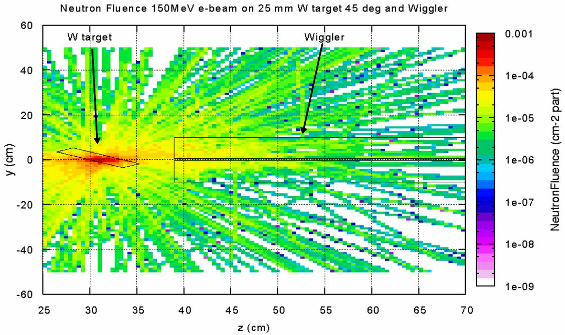
Fig. 10. Neutron fluence in the case 25 mm W target.
