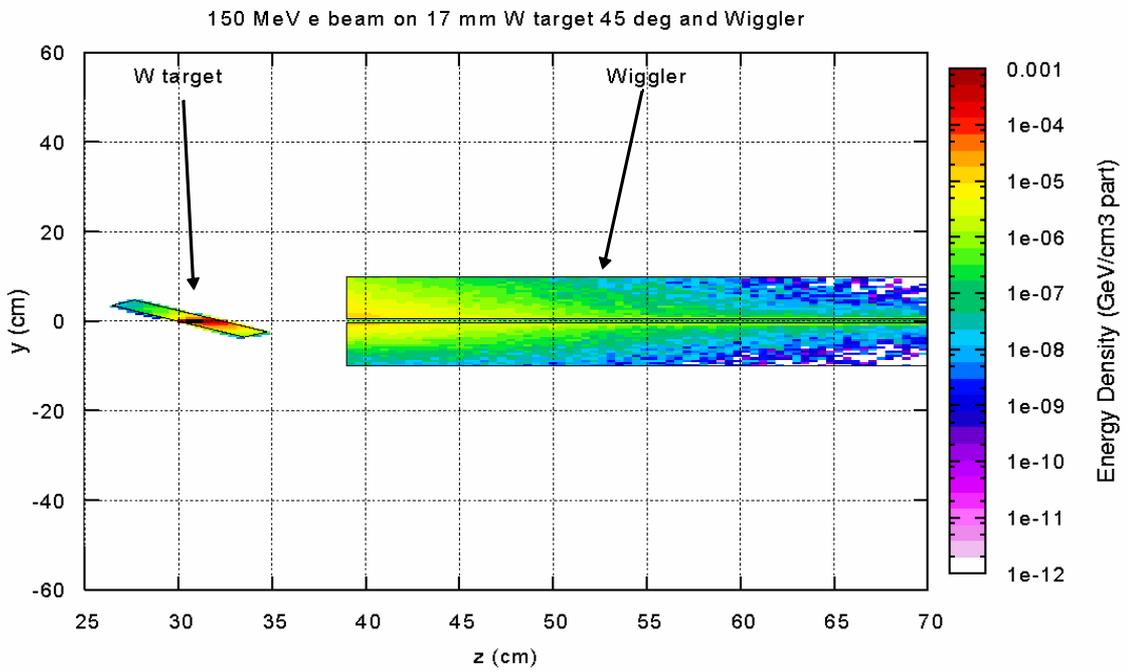
Fig. 5. Energy density deposition in the 17 mm W target and in the wiggler.
