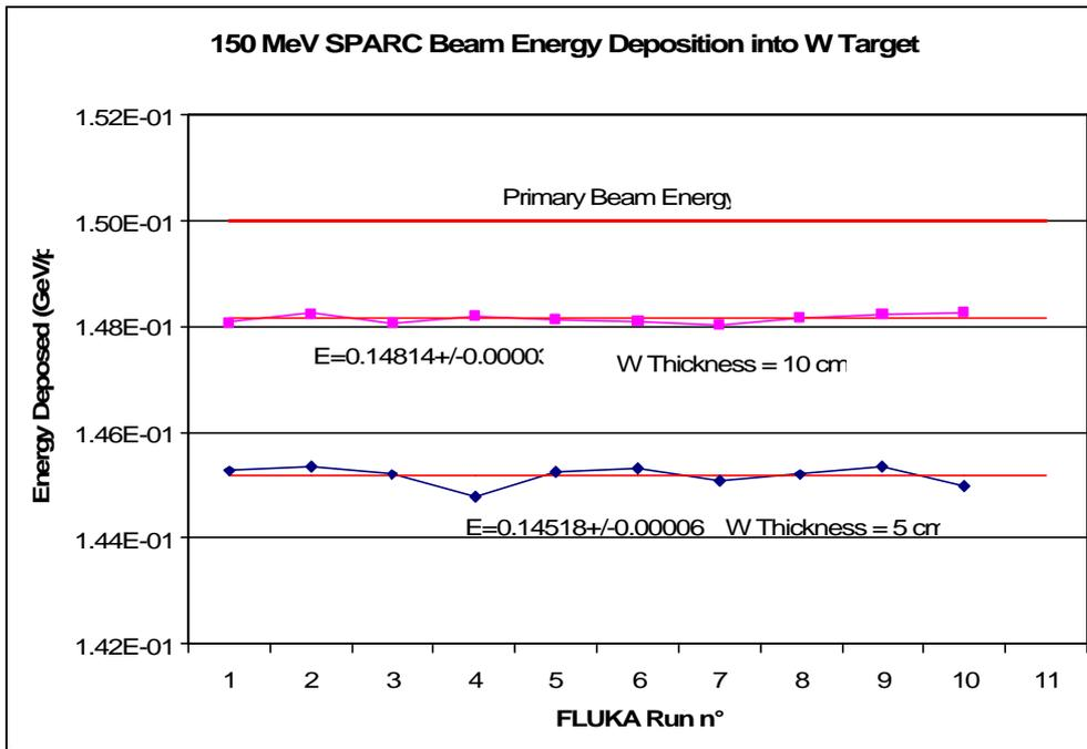
Fig. 2. Absorption of the SPARC beam in W , 10 FLUKA runs.
