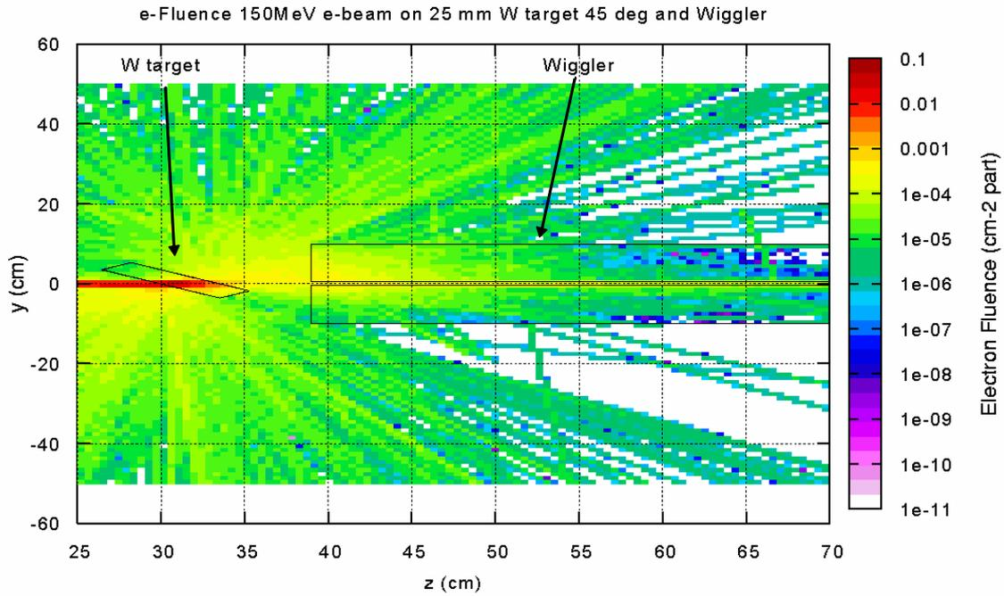
Fig. 6. Electron fluence in the case of 25 mm W target.
