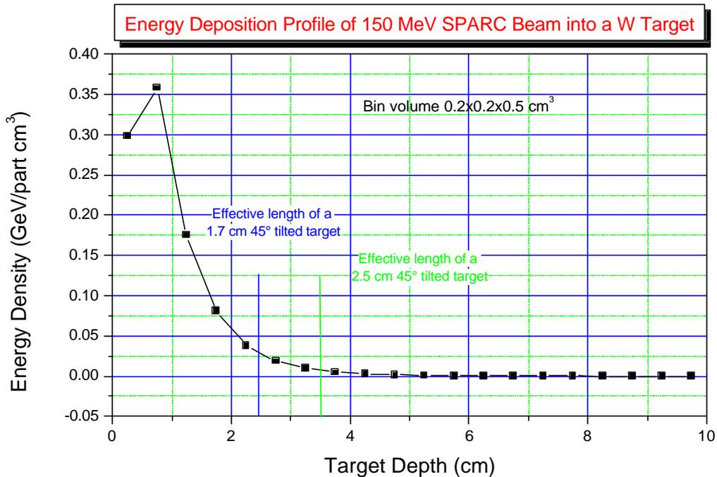
Fig. 3. Energy deposition vs. target depth.
