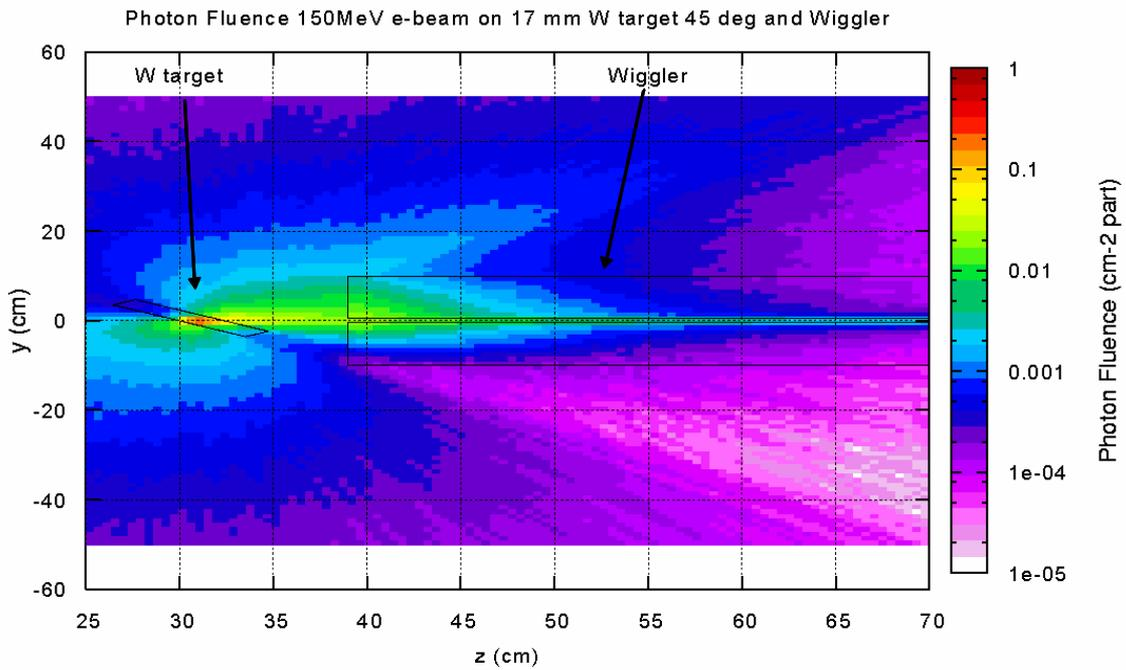
Fig. 9. Photon fluence in the case 17 mm W target.
