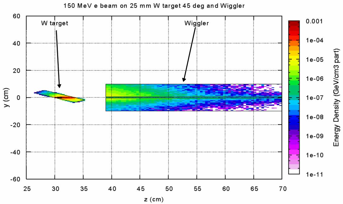
Fig. 4. Energy density deposition in the 25 mm W target and in the wiggler.
