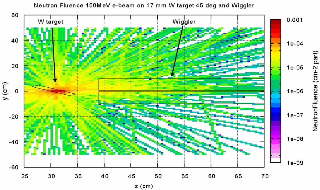
Fig. 11. Neutron fluence in the case 17 mm W target.
