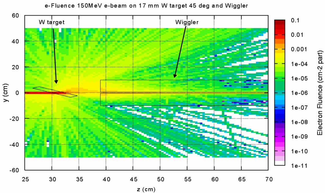
Fig. 7. Electron fluence in the case of 17 mm W target.
