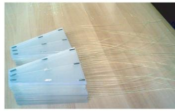
1 cm scintillator tiles (Protvino), each read by 3 wavelength shifting fibers (Bicron, 1mm) 36 fibers/sector, 1 photomultiplier/sector
