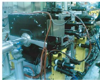
The four half-calorimeters installed around the DAFNE interaction region
