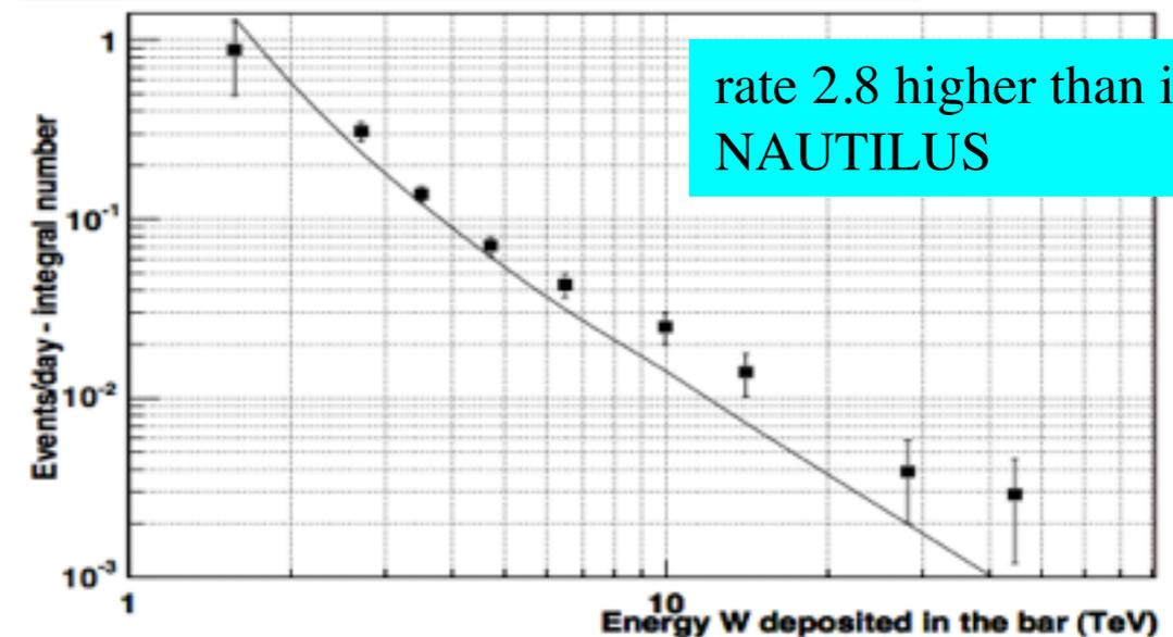
Fig. 11. EXPLORER 2003-2006 : The integral distribution of the event rate after the background unfolding, as in Fig.5, compared with the expected distribution (continuous line). The prediction is computed using Table 1 multiplied by a factor 2.8 (see text).
