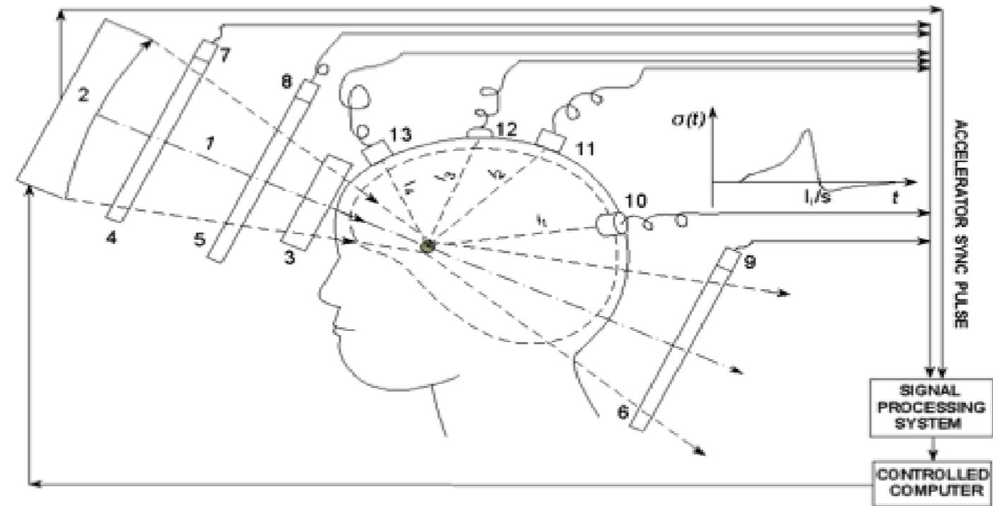
Figure 1: Scheme of radiation- acoustic monitoring of therapeutic beam in patient's body-
