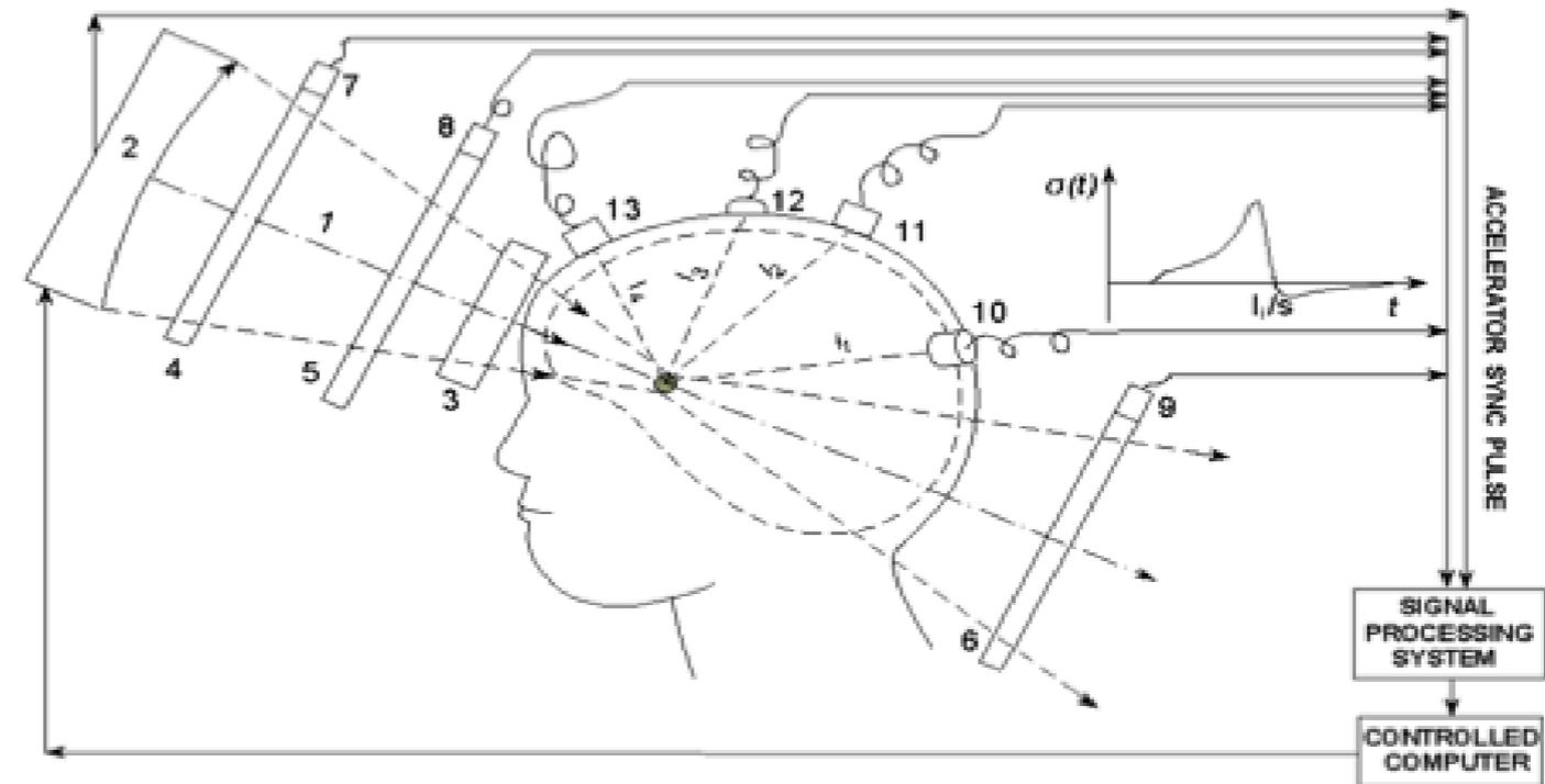
Figure 1: Scheme of radiation- acoustic monitoring of therapeutic beam in patient's body-
