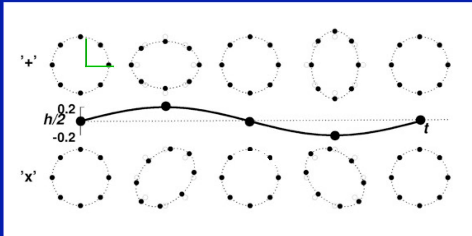
Detectors are sensitive to the polarization and to the angle of incidence
