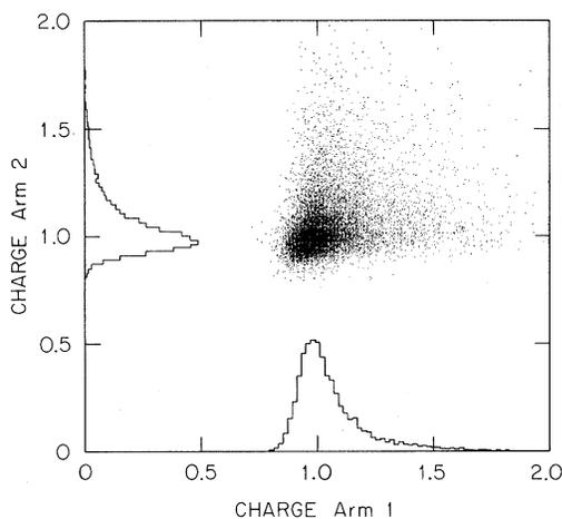
FIG. 2. A scatter plot of the measured charge in each arm of the detector for two-prong events. The charge measured in each arm of the detector is projected into a histogram illustrating the overall charge resolution. There are about 13 000 events in the figure.
