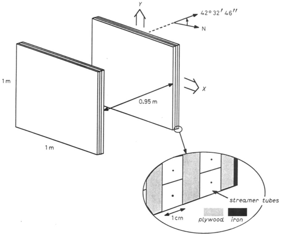
Fig. 1. - Experimental set-up.
