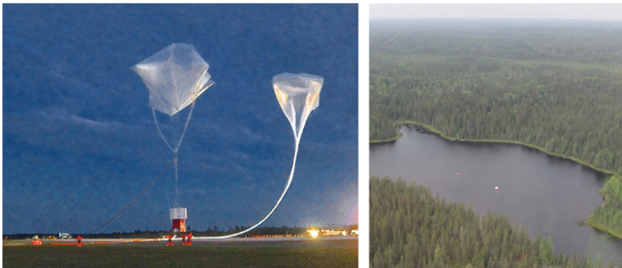
Fig. 8 Left: Timmins (Ontario, Canada) Stratospheric Balloon Base, August 25, 2014, 0:53 UT: the perfect launch of EUSO-Balloon by the balloon division of the French Space Agency CNES, the auxiliary balloons (above the payload in the picture) warrant a smooth launch even in case of moderate surface winds. Right: the instrument floating in the middle of "Lake Euso" after splashing down at 8:59 UT. All systems survived the impact and more than eight hours in the water thanks to a dedicated "water-landing" design
