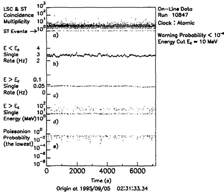
Fig. 1. The display of the PHRASE supernova monitor program. LSC means 'Liquid Scintillation Counter' and ST 'Streamer Tubes'.
