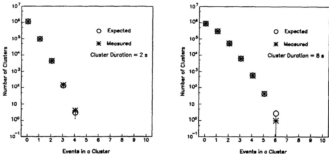
Fig. 4. Observed and predicted number of event clusters vs. cluster multiplicity for time intervals of 2 s (left) and 8 s (right) during the one-year monitoring period. A similar plot for the ERP system also indicates no deviation from the Poisson expectation.
