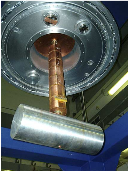
Fig. 2. The suspended bar in the opened cryostat.
