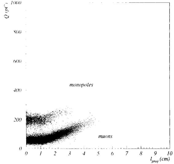
Fig. 7. Mean charge for a sample of muons and for simulated monopoles as a function of projected track length. A cut can be applied to discriminate monopoles with  $\beta > 5 \times 10^{-3}$  with high efficiency and a small muon contamination.
