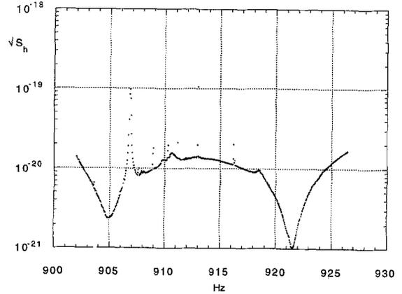
Fig. 1. Sensitivity to stochastic gw background with SNR = 1 for EXPLORER.  $T = 2.9$  K,  $M = 2300$  kg,  $Q = 10^6$ , average spectrum over 31.4 days (1991).
