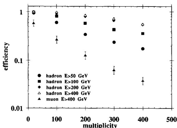
Fig. 10. Detection efficiency as a function of multiplicity cut.
