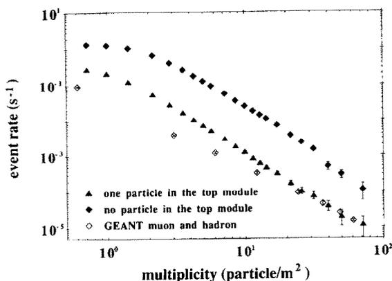
Fig. 12. Measured single particle rate in the bottom module.
