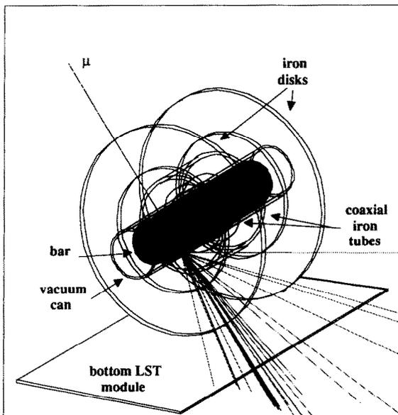
Fig. 6. Simulated interaction of a 1-TeV muon in the detector.
