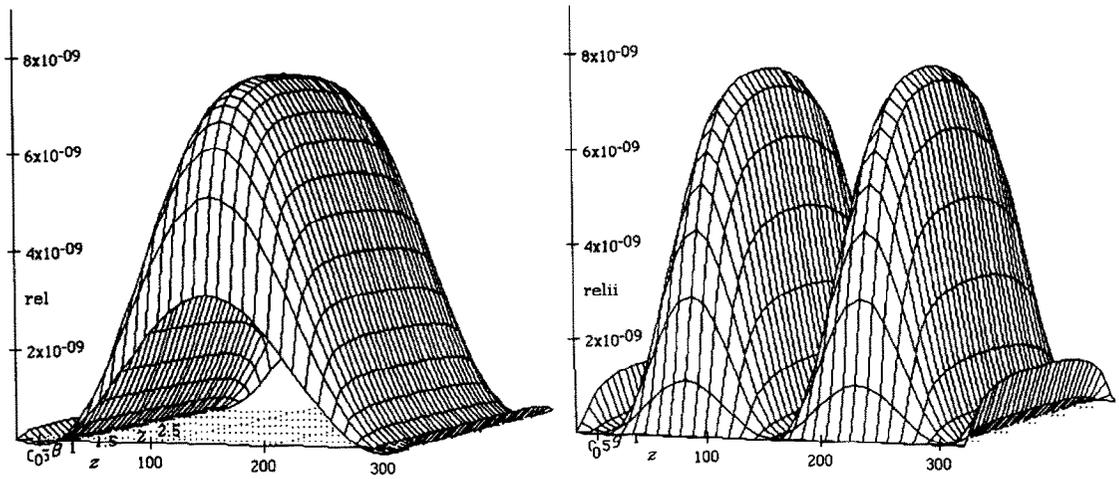
Fig. 5. Harmonics response as a function of the impinging particle angle and point.
