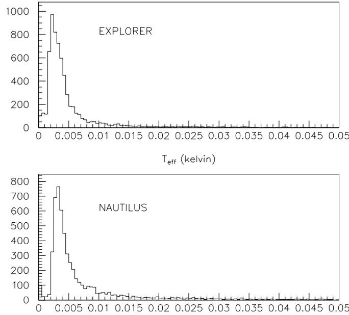
**Figure 2.** The distributions of the hourly averages of  $T_{\text{eff}}$  in kelvin units for EXPLORER and NAUTILUS. We accept only the time periods with hourly averages  $\overline{T_{\text{eff}}} \leq 10$  mK.
