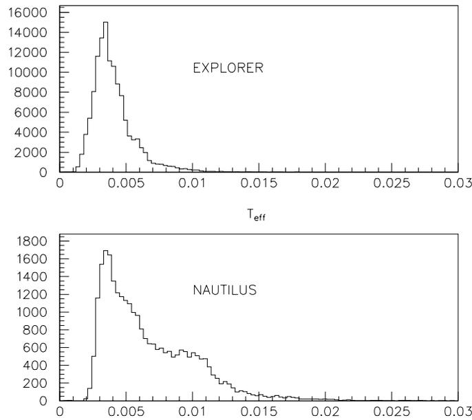
**Figure 3.** The distributions of the 10 min averages of  $T_{\text{eff}}$ , before each event, in kelvin units for the EXPLORER and NAUTILUS events (with hourly  $\overline{T_{\text{eff}}} \leq 10$  mK). We accept only the events with the 10 min average  $T_{\text{eff}} < 7$  mK. Note that the EXPLORER events are more numerous than the NAUTILUS events because of the different bandwidth.
