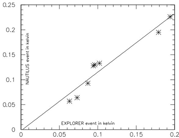
**Figure 8.** Correlation between the event energies of NAUTILUS with those of EXPLORER for the eight coincidences that occurred in the sidereal hour interval 3 to 5, in time periods  $\geq 1$  h. The correlation coefficient is 0.96. No energy filter was applied.
