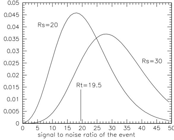
**Figure 1.** Differential probability that the event has the signal-to-noise ratio shown on the abscissa when the signal has  $R_s = 20$  (near the threshold  $R_t = 19.5$ ) and  $R_s = 30$ .
