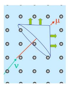
**Figure 5.11:** Neutrino telescopes consist of large arrays of photomultiplier tubes underwater or under ice. They detect the Cherenkov light emitted by charged particles which have been produced in neutrino interactions – here from an up-going muon which stems from a neutrino having crossed the Farth.
