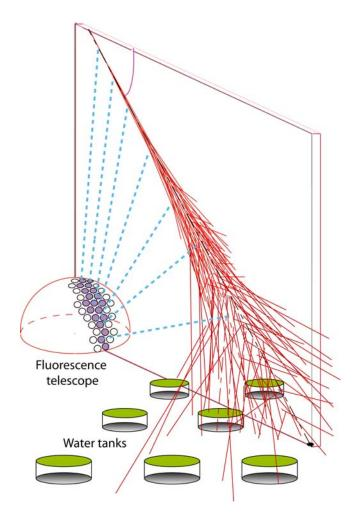
**Figure 5.7:** The Auger detection principles: Optical detection of fluorescence light from air showers recorded by telescopes particles at ground level recorded by Cherenkov water tanks.
