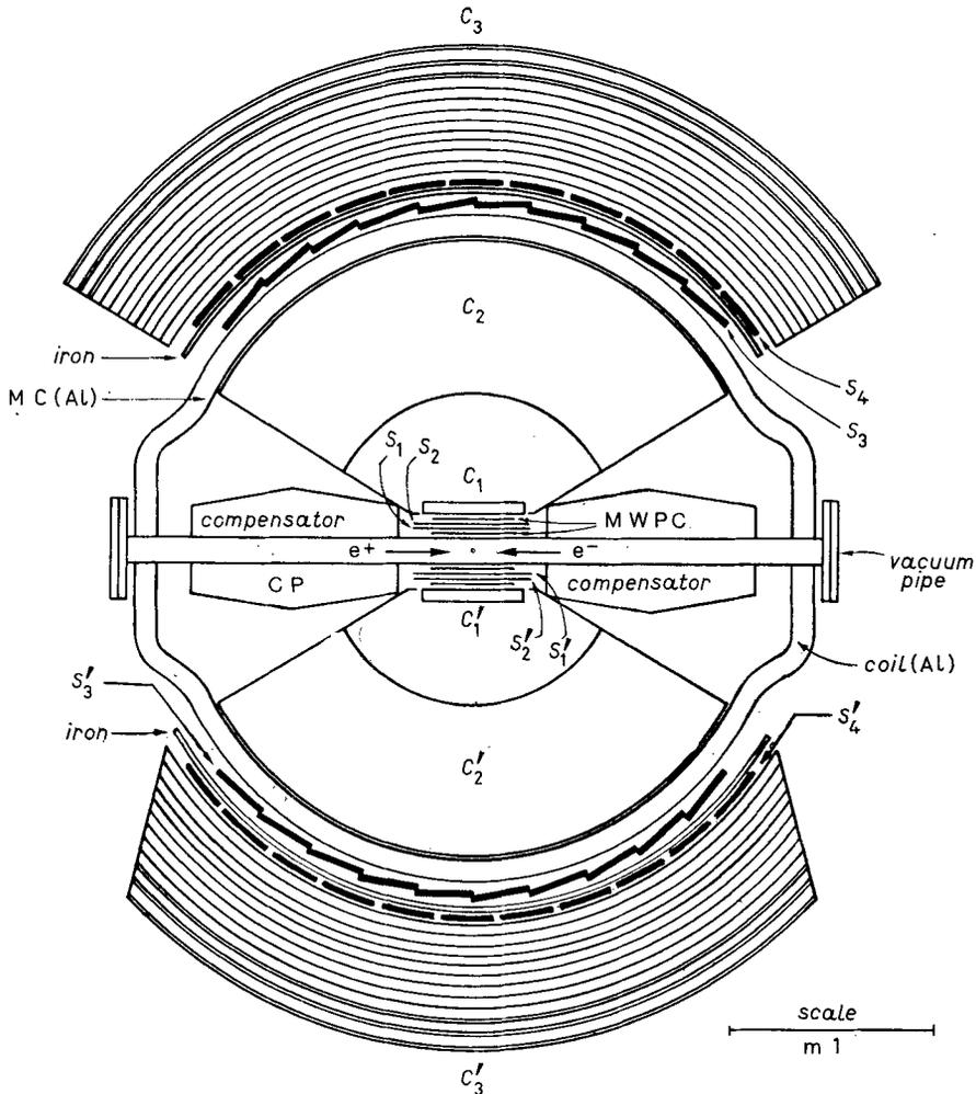
Fig. 1. - Vertical section of the experimental apparatus:  $C_1, C_1'$  are narrow-gap spark chambers;  $C_2, C_2'$  wide-gap cylindrical spark chambers for momentum analysis;  $C_3, C_3'$  thick-plate spark chambers for particle identification; MWPC multiwire proportional chambers;  $S_1, S_2, \dots, S_4'$  scintillation counters.
