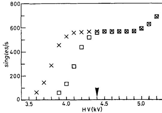
Fig. 3. - Singles counting rate for the streamer tubes for isotropic electrons ( $^{90}\text{Sr}$ ) and single photoelectrons. Starting from  $\sim 4.4$  kV, single electrons are detected with practically full efficiency and without spurious pulse detection.  $(3 \times 3)$  cm $^2$ , 60  $\mu\text{m}$ , He+n-pentane, 3:1.  $\times \beta$ ,  $\square$  single electron.
