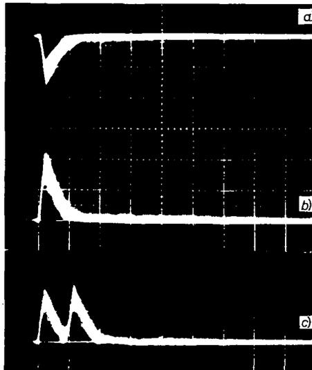
Fig. 4. - The horizontal scale is 100 ns/div. In the last case the reflection from the nonterminated end is visible. No attenuation is seen after  $\sim 30$  m propagation, indicating no problems with these dimensions: a) wire pulses at 4.4 kV, 50 mV/div; b) induced pulses on a 1 m long  $x$ -strip, 20 mV/div, 100  $\Omega$  terminator; c) induced pulses on a 15 m long  $d$ -strip ( $30^\circ$  with respect to the wires), 10 mV/div, 50  $\Omega$  terminator.
