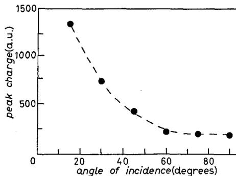
Fig. 6. - Streamer pulse height *vs.* the angle of the track with respect to the wire, as measured with cosmic rays. For a given streamer dead region length (fixed by the gas mixture) the pulse height is a measure of the track projection along the wire.  $(3 \times 3)$  cm<sup>2</sup>,  $60 \mu\text{m}$ ,  $\mu$ , He+n-pentane, 3:1, 4.4 kV.
