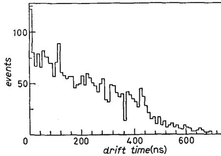
Fig. 5. - Drift time distribution for the streamer tubes as measured with cosmic rays. The distribution is that expected given the geometry of the cell. The resulting time accuracy is  $\sim 150$  ns.  $(3 \times 3)$  cm<sup>2</sup>,  $60 \mu\text{m}$ ; He+n-pentane, 3:1, HV = 4.4 kV.
