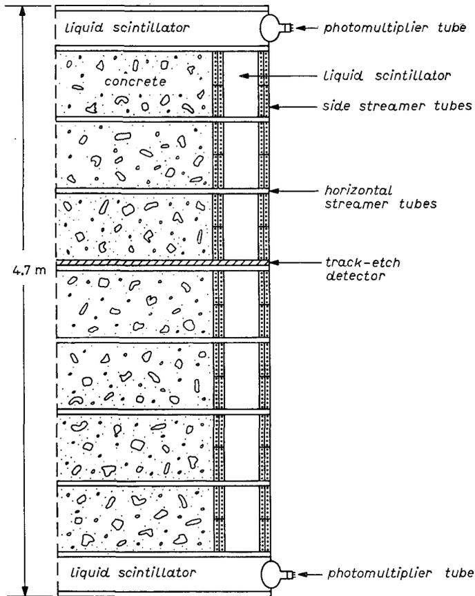
Fig. 2. - Cross-sectional sketch showing the active components which close the sides of the detector.
