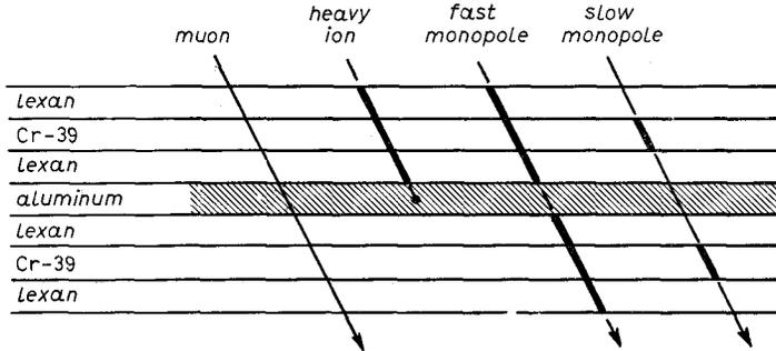
Fig. 6. - The concept of monopole detection in the track-etch detector.
