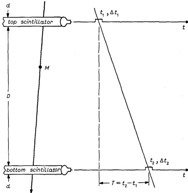
Fig. 4. - The concept for slow particle detection in the scintillator system is shown. A long pulse due to the slow passage of the particle is observed in both the top and the bottom layers.
