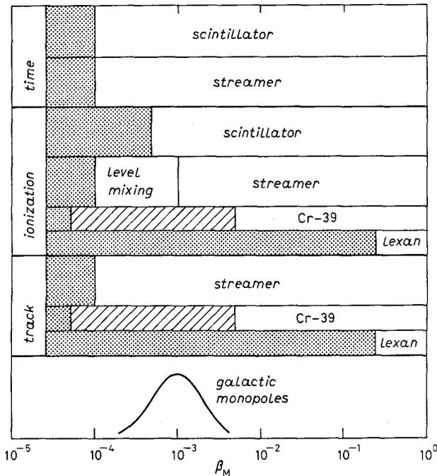
Fig. 7. - Summary of the response of the various detector elements for monopole detection.
