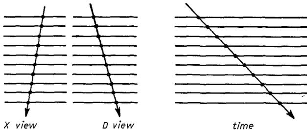
Fig. 5. - The concept of monopole detection in the streamer tube system is shown. A track in space is observed, with a linear distribution in time of the ten streamer tube hits (time track).
