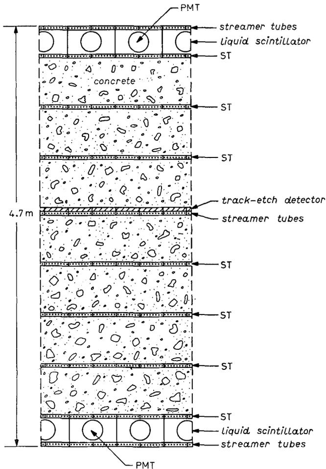
Fig. 1. - Cross-sectional sketch of the detector, showing the relative position of the various components.
