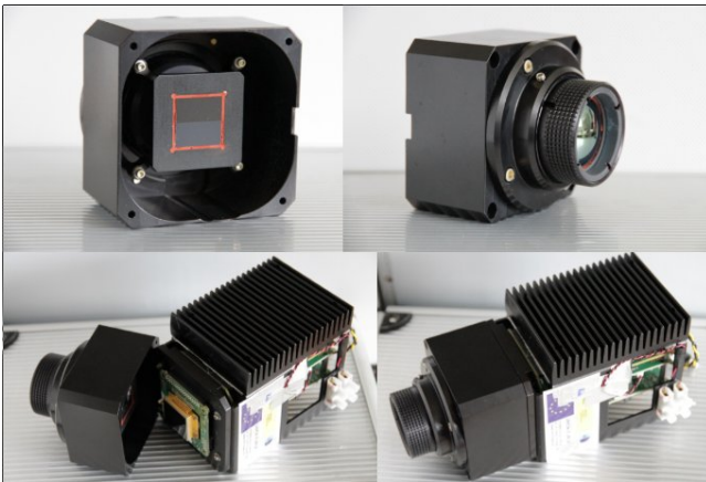
Figure 4: Breadboard model manufactured at INTA facilities for the Infrared Camera of JEM-EUSO.
