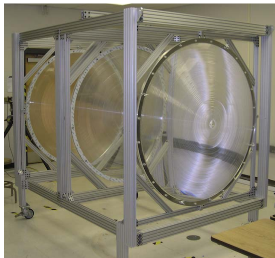
Figure 1: The bread board model (BBM) of the JEM-EUSO optics. The lens diameter is 1.5 m.
