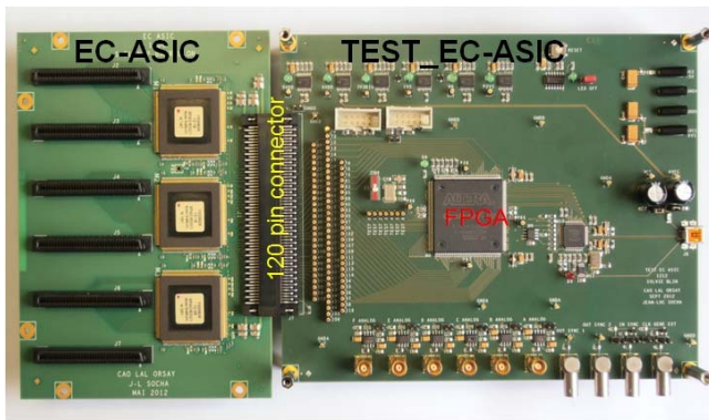
Figure 10: Picture of the ASIC prototype board connected to a dedicated test board.
