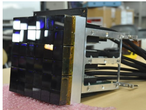
Figure 2: The full focal surface of EUSO-TA consisting of one PDM.
