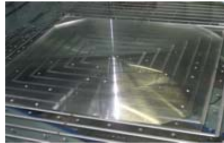
Figure 5: A photo of the TA-EUSO front lens on the machine after manufacturing.
