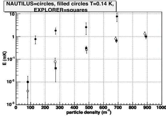
Figure 2. Averages of signals with energy  $E_{exp} \leq 0.1 K$ , grouping data in ranges of particle density  $\Lambda$ . Filled circles NAUTILUS at  $T = 0.14 K$ , open circles NAUTILUS at  $T = 3 K$ , filled squares EXPLORER at  $T = 3 K$ . The data gathered at  $T = 0.14 K$  are almost one order of magnitude larger than those collected at  $T = 3 K$ .
