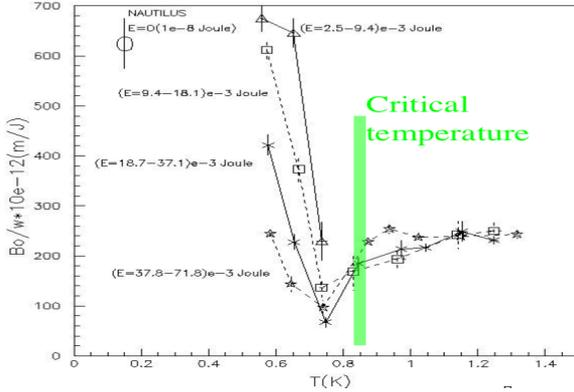
Figure 1. RAP results : the amplitude of the first longitudinal mode normalized to the electron beam absorbed energy as function of the temperature  $T$  and for different ranges of the absorbed energy. This ratio is a constant for normal conducting aluminum but has a complicated behavior for super conducting aluminum.
