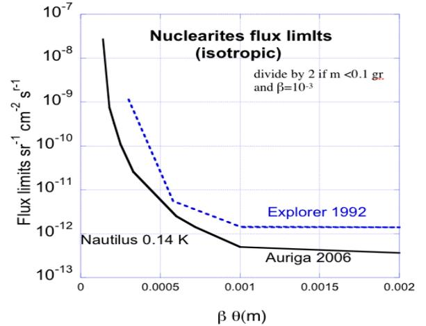
Figure 5. Nuclearites flux upper limits from gravitational wave bar detectors. Other detectors have much better sensitivities, but the detection techniques are completely different. The bar detectors are like "calorimeters" for this search
