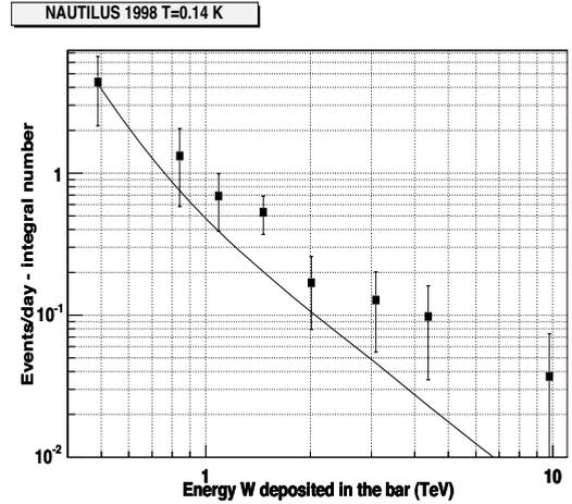
Figure 3. NAUTILUS 1998. The integral distribution of the event rate after the background unfolding, compared with the expected distribution (continuous line). The prediction is computed using the data of Table 1 and using the appropriate value  $\alpha_s = 3.7$ .
