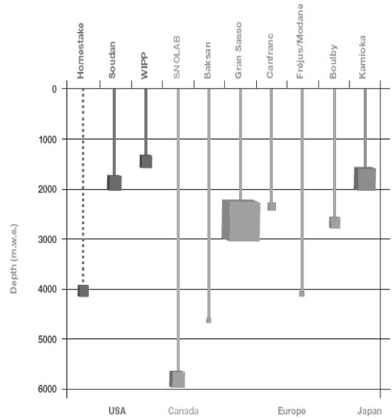
Figure 1. Depth (in meters of water equivalent) and space of the experimental halls of underground laboratories in the world. The Gran Sasso is the largest having in total 18000 m<sup>2</sup>
