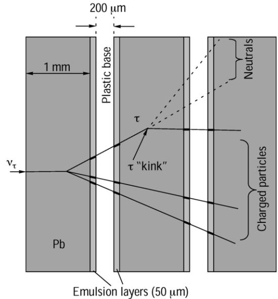
Figure 3. OPERA: the  $\tau$  detection principle in the lead foils - nuclear emulsions sandwich (brick)
