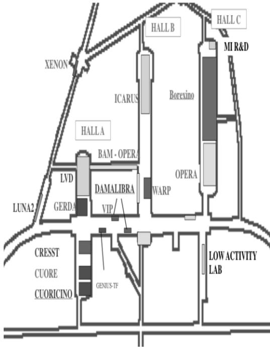
Figure 2. The three Gran Sasso Laboratory experimental halls and the space allocation. Some smaller experiments are located in the service tunnels
