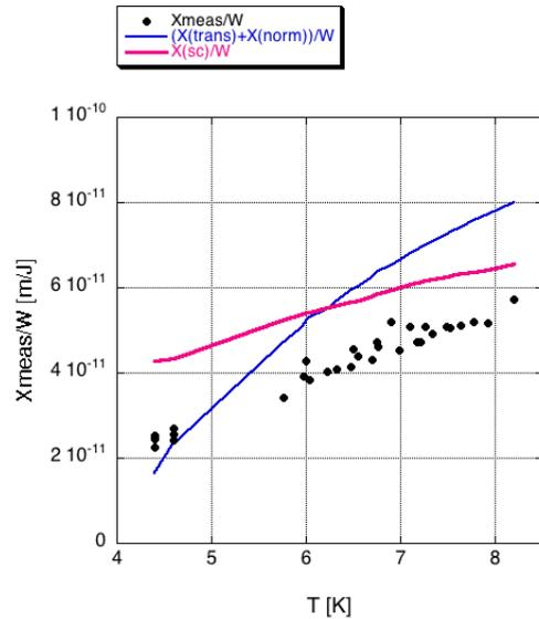
Figure 6. Line: maximum amplitude normalized to the energy lost by the beam evaluated respectively with the superconducting parameters (thick-line) and with the normal ones (taking into account also the transition) (thin-line) vs Temperature. Dots: observed values
