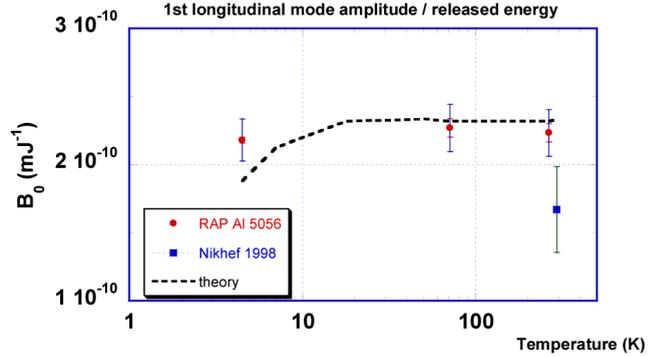
Figure 2. Maximum measured amplitude of the 1st longitudinal mode normalized to the deposited energy vs. Temperature.
