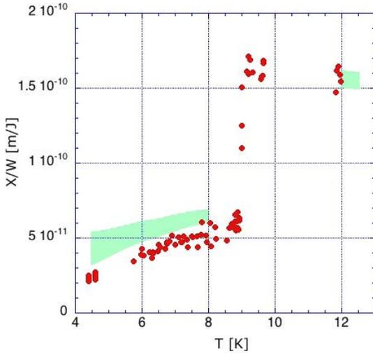
Figure 5. 1st longitudinal maximum amplitude normalized to the total energy lost per beam pulse ( $W$ ) vs. Temperature ( $T$ ). Dots: measured values. Light green bands: expected values from thermophysical data for pure Nb in the n state ( $9 < T < 12K$ ) and in s state ( $T < 9K$ ) with their error bars.
