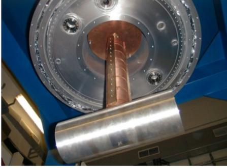
Figure 1. Al5056 cylinder and its suspension system.
