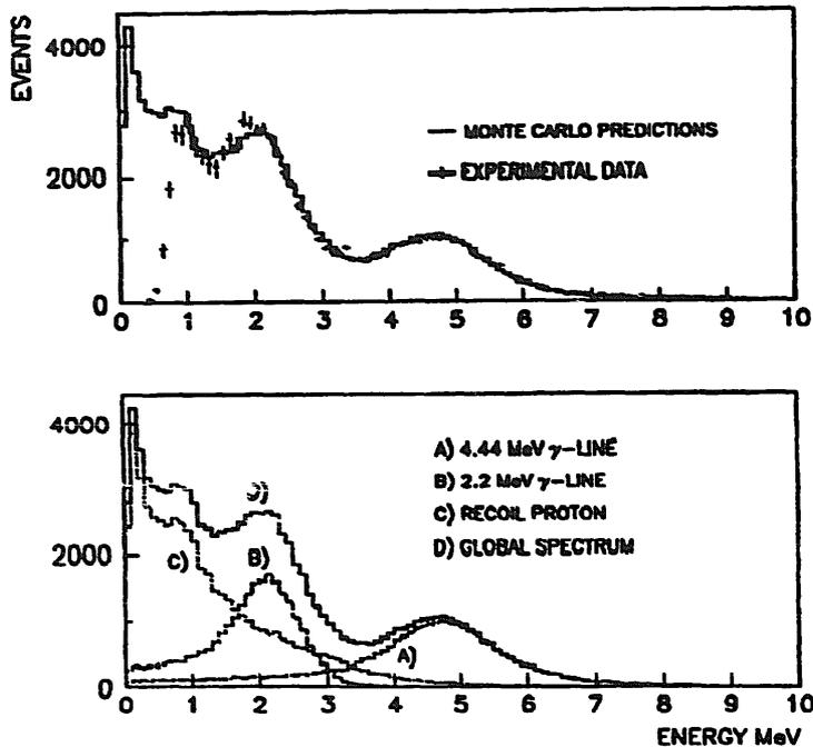
Fig. 1. a) Energy spectrum for events from the Am/Be source. The 4.44 and the 2.2 MeV  $\gamma$ -lines are visible. The histogram is a Monte Carlo simulation. b) The decomposition of the Monte Carlo global result into different contributing processes.
