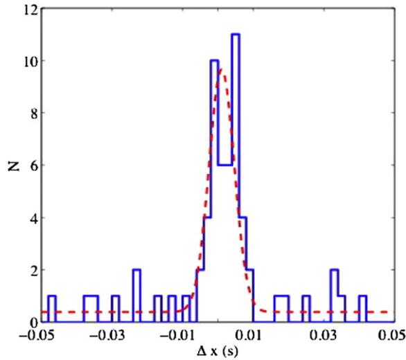
Figure 4. Distribution of time differences between events in coincidence at the antenna output (EXPLORER) and in the cosmic rays detector. We expected for the coincidences a Gaussian distribution over a flat background due to noise not correlated to the cosmic rays events. The Gaussian fit yields for the coincidences an average instrumental systematic delay  $\Delta t_0 = 1.3$  ms and a standard deviation (on a single detector)  $\sigma = 3.6$  ms.
