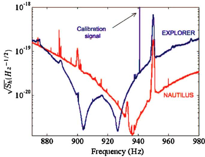
Figure 1. Typical present sensitivity curve for EXPLORER and NAUTILUS detectors.
