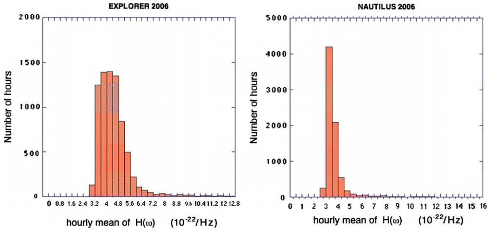
Figure 3. Histograms of the noise level of EXPLORER and NAUTILUS, averaged over 1 h, in the year 2006.
