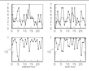
**Figure 11.** The 1998 data with energy filter. The upper graph on the left shows the number of coincidences  $n_c$  indicated by asterisks and the average number  $\bar{n}$  of accidentals versus the sidereal hour. The lower graph on the left shows the Poisson probability of obtaining a number of coincidences greater than or equal to  $n_c$ . The two graphs on the right show the result using the solar time in hours.
