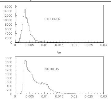
**Figure 3.** The distributions of the 10 min averages of  $T_{\rm eff}$ , before each event, in kelvin units for the EXPLORER and NAUTILUS events (with hourly  $T_{\rm eff} \leqslant 10\,{\rm mK}$ ). We accept only the events with the 10 min average  $T_{\rm eff} < 7\,{\rm mK}$ . Note that the EXPLORER events are more numerous than the NAUTILUS events because of the different bandwidth.
