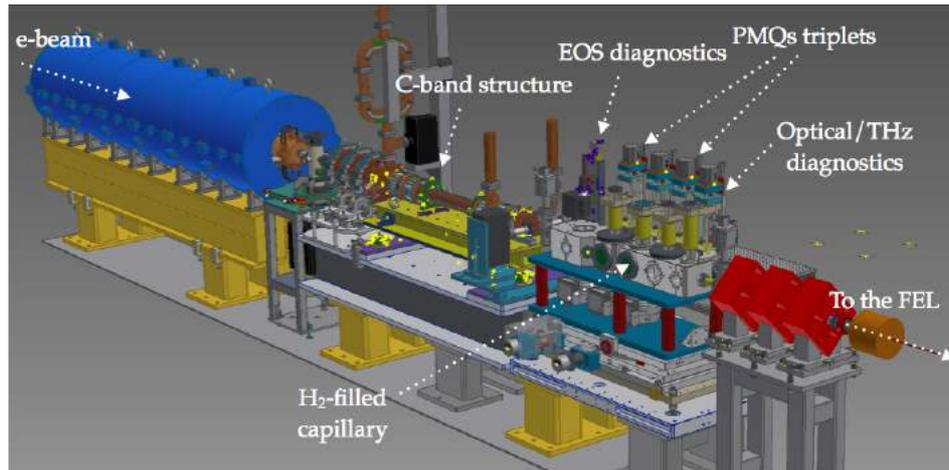
**Figure 12** - Update layout of the photo-injector. The third S-band structure has been replaced by a C-band structure and the plasma interaction chamber, fully equipped with beam and plasma diagnostics and permanent quadrupole magnets.
