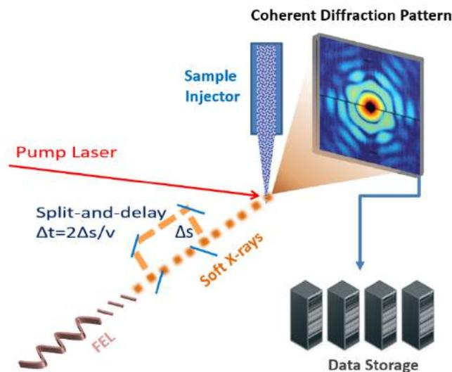
**Figure 10** - Simplified layout of an imaging experiment using the EuPRAXIA@SPARC\_LAB FEL.
