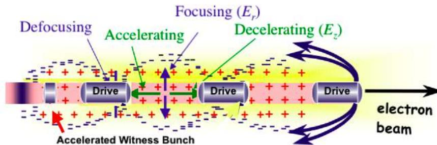
Figure 9: Multibunch excitation of a plasma wave
