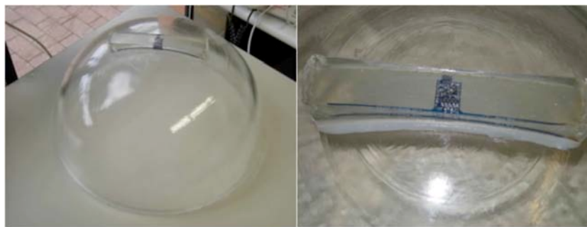
Figure 3 – The WISP glued to the sphere.
