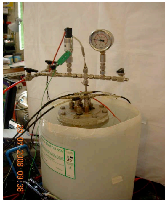
Figure 4. The pressurized experimental cell surrounded by a large water bath.
