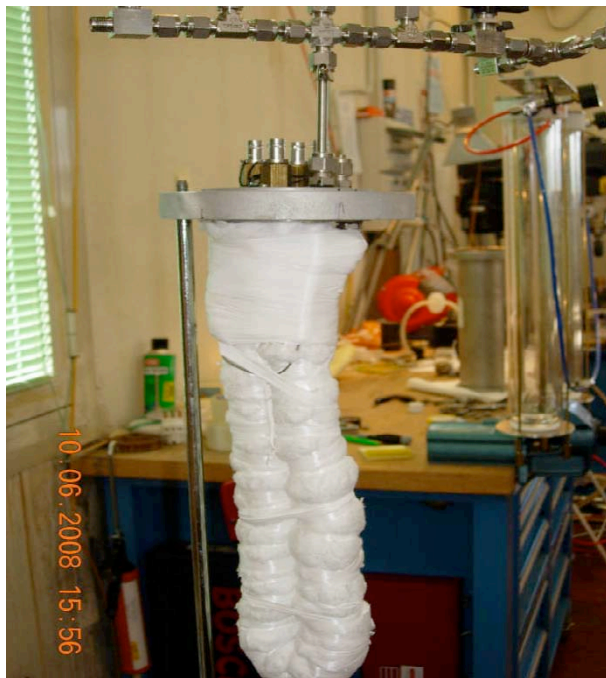
Figure 3. The braid placed inside thermal insulation.
