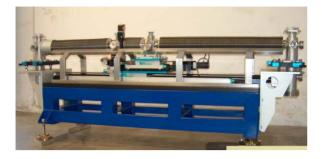
Figure 5: Emittance-meter device with long bellows.
