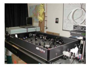
Figure 3: HIDRA-50 amplifier for the SPARC laser.
