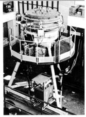
Fig. 4. Finished shells of Y-magnets at each end of interaction region.
