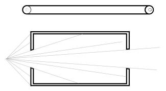
Figure 3: How to make a very thin light beam.
