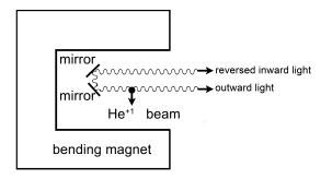
Figure 2: Device aimed at comparing light beams which leave perpendicularly to the orbit in opposite directions.
