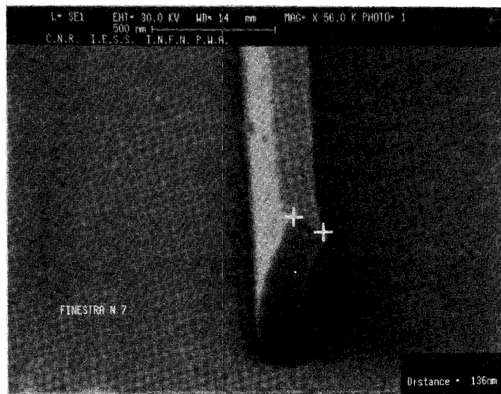
Fig.1. Replica of a 0.15 µm wide structure on PMMA resist.
