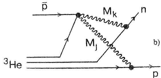
FIG.1 - Diagrams describing the two-step mechanism of the reactions  $\bar{p}d \rightarrow \pi^- p$  (a) and  $\bar{p}^3\text{He} \rightarrow pn$  (b).  $M_j$  and  $M_k$  are the effective mesons (or glueballs) exchanged after the initial  $\bar{p}p$  annihilation.
