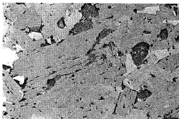
FIG. 1 - Microscope picture of YBCO crystals observed in polarized light (—— = 40 \mu\text{m} ).
