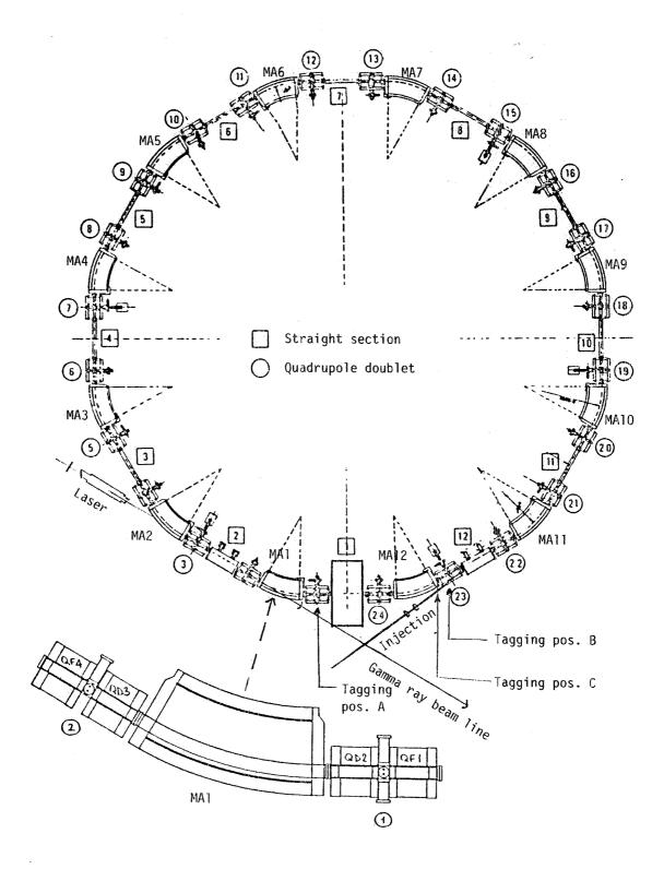
$\overline{\text{FIG. 1}}$  - A schematic representation of the layout of the Adone storage ring with an indication of the electron-Laser interaction region, the direction of the gamma ray beam and positions A,B and C of the tagging detectors.
