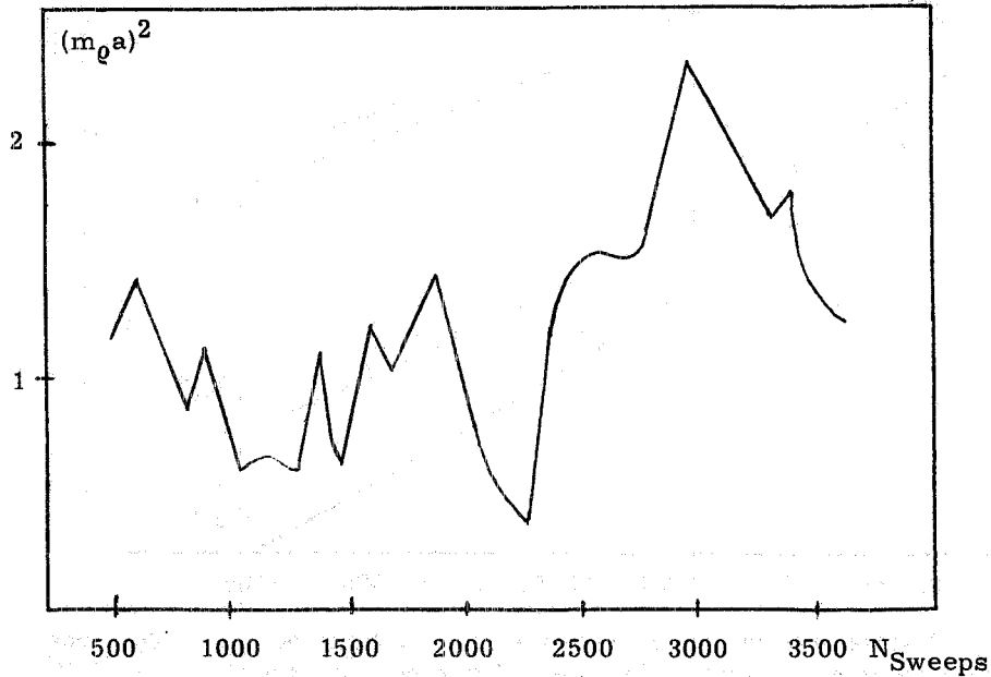
FIG. 4 - The squared mass of the \rho -meson time the lattice spacing a at K=0.1475 as a function of the total number of Montecarlo sweeps. Analogous curves could be drawn for the other particles.
