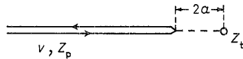
Fig. 1.1. – Projectile Z_p approaching the target Z_t with the relative velocity v moving in a head-on collision.
